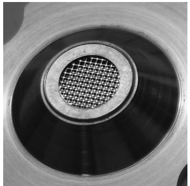
Fig. 9. The extraction electrode with the new fine double grid configuration. The diameter of the grids are 4.5 mm, the distance between the two grids is 0.4 mm.
